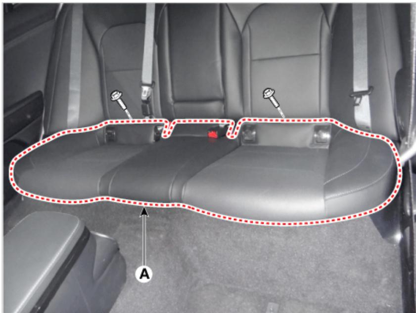
2. Remove the rear seat cushion after disconnecting the heater connector (A).
